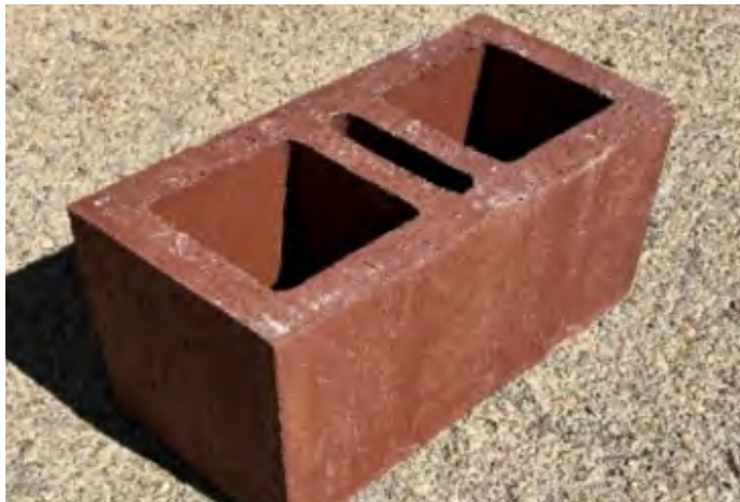
Figure 3 Hollow Clay Units (Left: 7 3/8" x 7 3/8" x 15 3/8", Right: 3 1/2" x 2 1/2" x 7 1/2", and 3 1/2" x 3 1/2" x 11 1/2")
