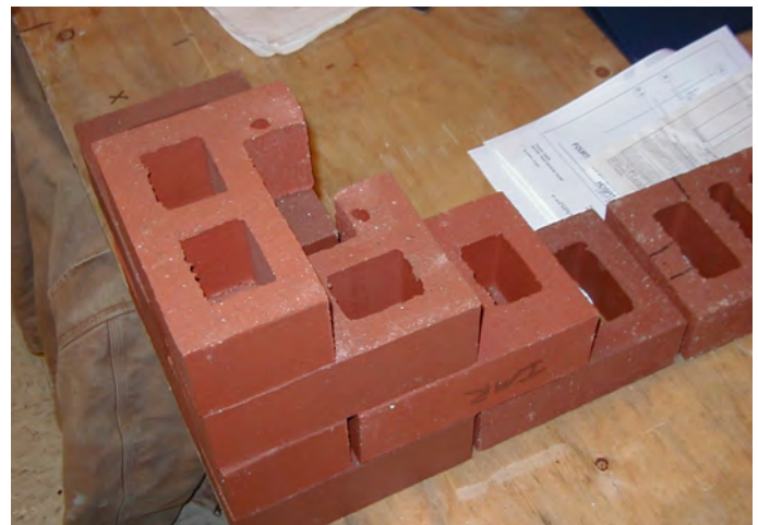
Figure 23 Custom Unit for a Four Inch Corner in a Six Inch Wall
