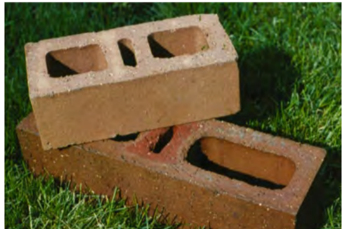
Figure 3 Hollow Clay Units (Left: 7 3/8" x 7 3/8" x 15 3/8", Right: 3 1/2" x 2 1/2" x 7 1/2", and 3 1/2" x 3 1/2" x 11 1/2")
